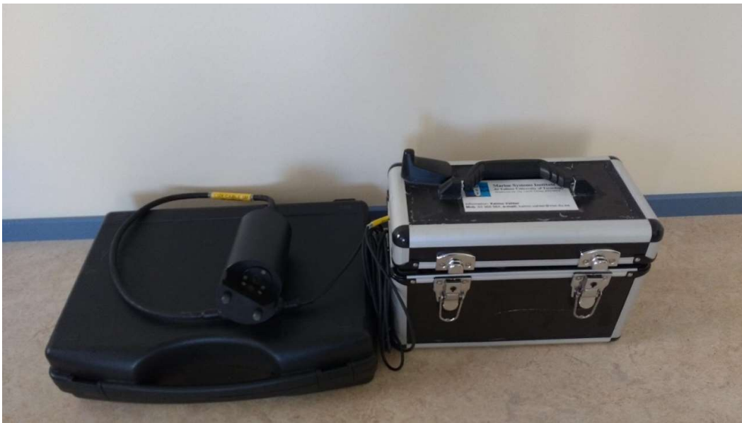
Figure 12 The UviLux sensor, integrated with portable modem/datalogger system and a battery, allowing autonomous operations both in field and lab
